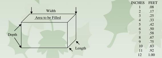
Multiply the length, width and depth (all in feet) of the area to be filled, then divide that by 27 cubic feet to get the total amount of cubic yards in the area you are filling.
